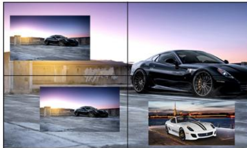
Image roaming: software processing can render any signal to a screen as a point,moving across the whole screen
